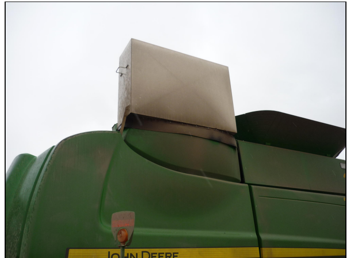
Figure 1. Metal air intake chimney created by Stelter Repair.
