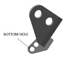
**Note:** In general, all rows will be set to the same hole. However, some rows may require unique settings. A typical example would be a row unit directly behind a tractor tire. In this example, this row unit should be set to exert more force on the row cleaner than the surrounding rows. If the system is normally operated in LIFT mode, install this row unit in the <u>bottom</u> hole. If the system is normally operated in the DOWN mode, install this row unit in the <u>top</u> hole.
