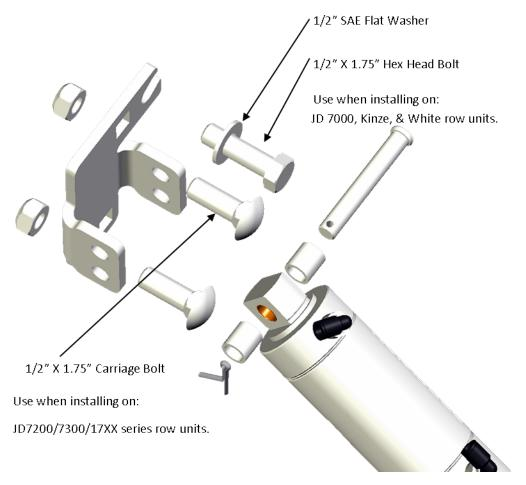
Install the base of the Cylinder to this bracket using the Cylinder Base Pivot Pin (755018). Use the two - 5/8" OD X 7/16ID X 0.688"L Spacer Bushings to properly secure and align the cylinder in the Base Mount Bracket.
