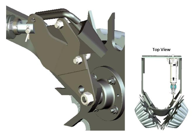
Secure the Rod Mounting Bracket to the clevis yoke on the cylinder using the supplied cylinder rod pivot pin (755019) and cotter pin. The default cylinder hole is the BOTTOM HOLE in the bracket.
