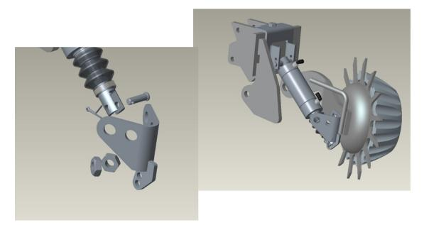
Secure the Rod Mounting Bracket to the clevis yoke on the cylinder using the supplied cylinder rod pivot pin (755019) and cotter pin.
