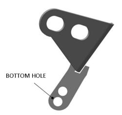
**Note:** In general, all rows will be set to the same hole. However, some rows may require unique settings. A typical example would be a row unit directly behind a tractor tire. In this example, this row unit should be set to exert more force on the row cleaner than the surrounding rows. If the system is normally operated in LIFT mode, install this row unit in the <u>bottom</u> hole. If the system is normally operated in the DOWN mode, install this row unit in the <u>top</u> hole.
