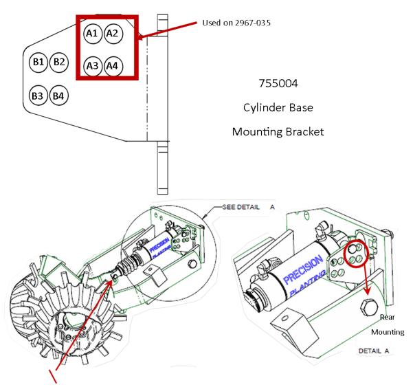
The hole used on the Rod Mount Bracket should correspond to the same hole used on the Base Mount Bracket. Example: Top to Top and Bottom to Bottom
