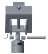
Tighten to 75 lb-ft of torque.
