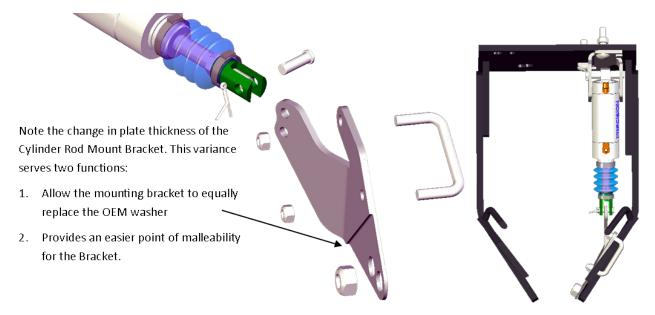
Secure the Rod Mounting Bracket to the clevis yoke on the cylinder using the supplied cylinder rod pivot pin (755019) and cotter pin. Refer to the Mounting Hole Selection guide at the end of this section for more information on which mounting holes to use with this bracket.
