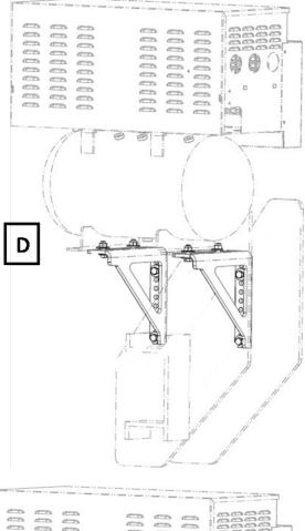
This mounting kit will be very similar to the previous mounting kit. The same brackets will be provided, however there will also be two U-bolts, removing the need for a drilling operation.
