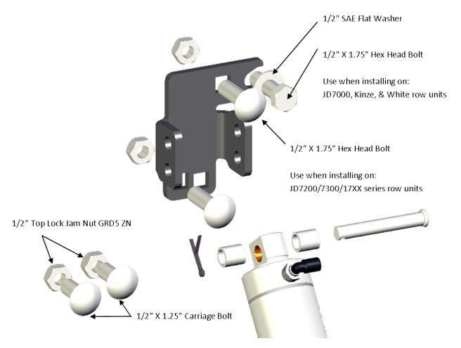
Install the base of the Cylinder to this bracket using the Cylinder Base Pivot Pin (755018). Use the two 5/8" OD X 7/16ID X 0.688"L Spacer Bushings to properly secure and align the cylinder in the Base Mount Bracket.
