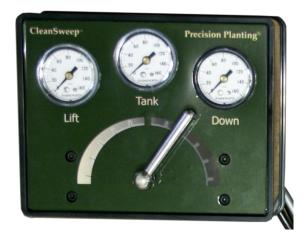
The amount of down or lift pressure that you use will depend on the specific row cleaners that are on the planter and the field conditions. It is not recommended that the row cleaner be used to move soil. Using a row cleaner for "tillage" or to move soil may result in uneven planting depth.
