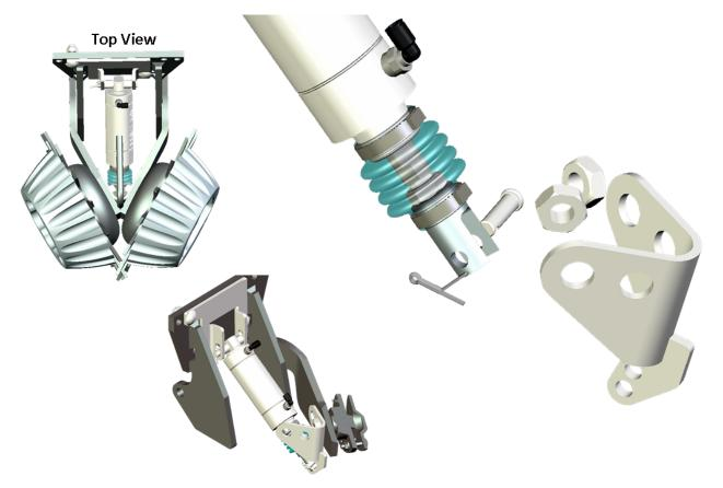
When installing the Cylinder Rod Mount Bracket, be sure it is properly aligned in the clevis yoke of the Rod and firmly seated in the curve of the row cleaner. This may require the exact angle of the bracket to be tweaked or modified in order to more perfectly match the individual row unit.
