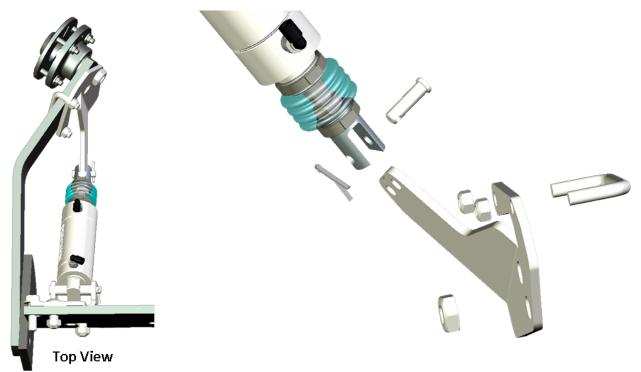
Secure the Rod Mounting Bracket to the clevis yoke on the cylinder using the supplied cylinder rod pivot pin (755019) and cotter pin. Refer to the Mounting Hole Selection guide at the end of this section for more information on which mounting holes to use with this bracket.
