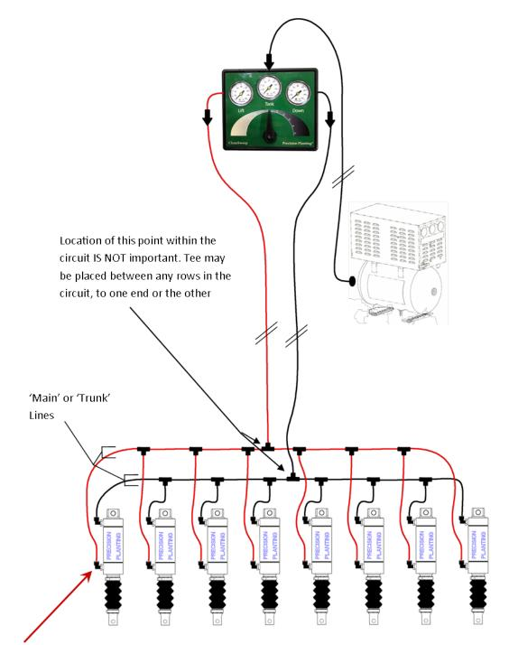
Note: the Lift Circuit line must be connected to the port towards the row cleaners (or rod portion of the cylinder)
