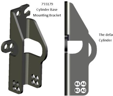
The default mounting position for the Cylinder base will be the bottom hole.
