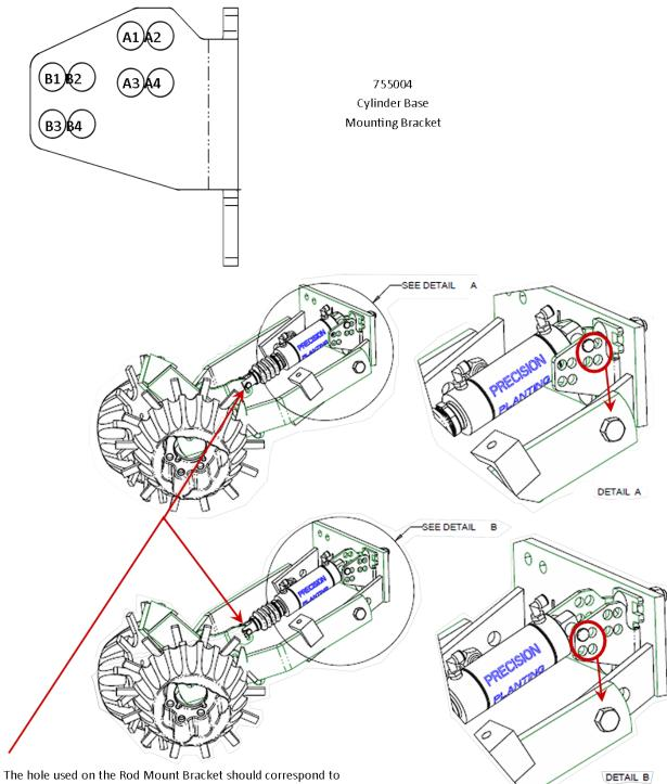
the same hole used on the Rod Mount Bracket should correspond to the same hole used on the Base Mount Bracket. Top to Top Bottom to Bottom
