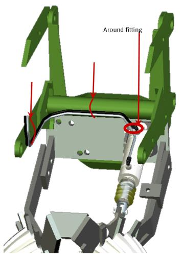
DO NOT pass the lines between the rear cylinder of the parallel arms and the row unit. This can act as both a pinch point and wear point.
