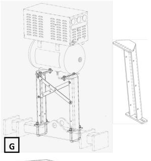
This mounting kit will locate the Compressor low and to the side of the main tongue. Used primarily for Kinze planters to provide clearance under the Lift and Twist transport. Two brackets, two U-bolts, and hardware will be supplied with this kit.
