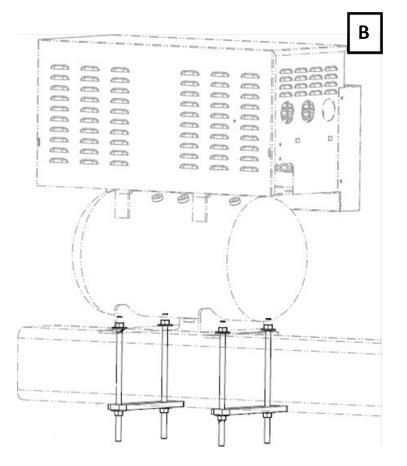
This group of mounting brackets will be most common on Kinze and stack-fold planters and may require the removal of the jack stand mounting bracket. Three U-bolts, three brackets, and the necessary hardware will be provided. Two of the brackets, similar to those shown below, will be used to space the tank above hoses and communication lines on the tongue or toolbar. The remaining U-bolt and bracket will be used to relocate the jack stand on Kinze planters to the vertical riser.
