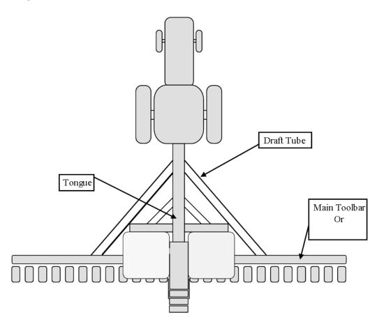
The diagram to the right will help identify possible mounting locations on your specific planter. Allow room for the lid to open properly. Measure 10" vertically and 8" to the rear of the point marked with an \*. The 'X' dimension is the spacing between the tank rail bolt holes, on center. The bolt holes are spaced 1" on center, with 1" slots at each end.
