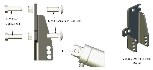
Tighten to 75 lb-ft of torque.
