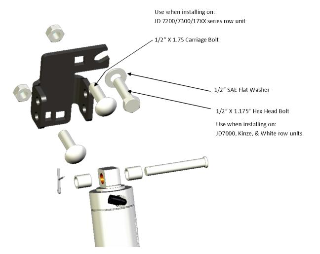
Install the base of the Cylinder to this bracket using the Cylinder Base Pivot Pin (755018). Use the 5/8" OD X 7/16ID X 0.688"L Spacer Bushing (towards the interior of the row) and the 5/8" OD X 7/16ID X 0.829"L Spacer Bushing (towards the exterior of the row) to properly secure and align the cylinder in the Base Mount Bracket.
