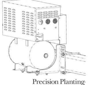
This mounting kit has the same concept as the basic U-bolt, that is adapted for non-standard tubes or channels that comprise the tongue of some planters.
