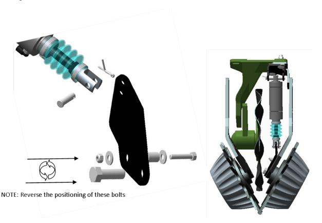
This will require removal of the existing 5/8" Bolt installed through the hub. When re-installing, re-use the existing 5/8" washer, ensure proper alignment of all components, and that the hub is firmly secured.
