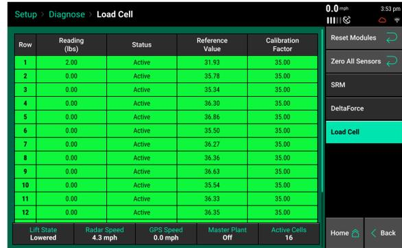
**Reading (lbs)** - displays the current weight that is being measured on each individual row.
