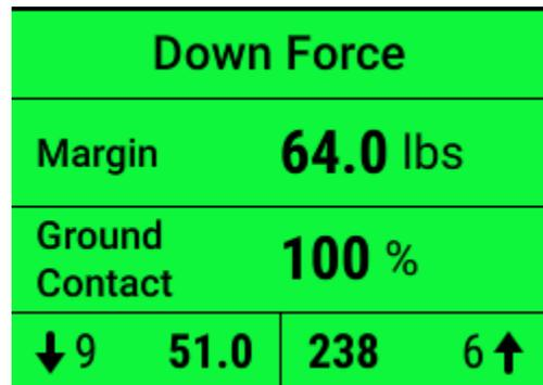
**Ground Contact**- The percentage of time the system can confirm that the gauge wheels have met the depth stop, which generally indicates that the row unit is planting at the depth to which it has been set. This is calculated by the percentage of time that the load cell is measuring 20 pounds or more.
