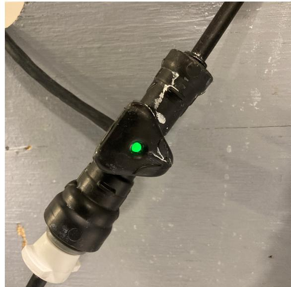
A red or orange light indicates the FlowSense is powered and the sensor is currently triggered, but not changing. This would indicate that the turbine to measure flow is NOT spinning. This could be due to no flow through the device, or foreign material is preventing the turbine from spinning.
