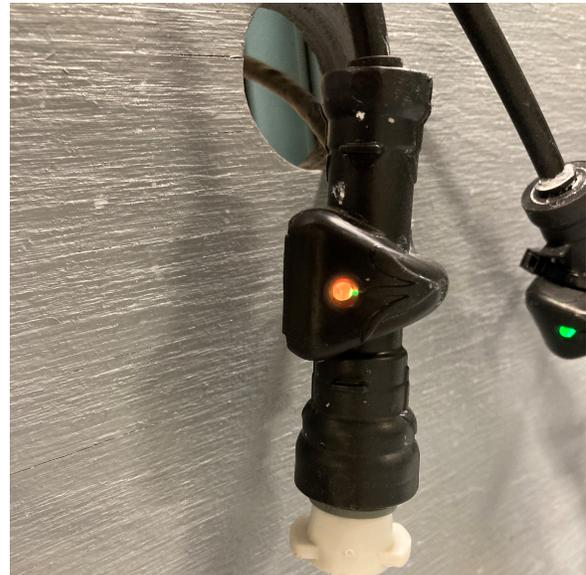
A yellow light or light that appears to be flashing rapidly indicates that the FlowSense is powered and the sensor is triggering on and off. This indicates that the FlowSense is measuring flow, therefore if there is flow currently, this is the CORRECT light color and is expected during normal operation.. The faster the light is flashing, the greater the amount of flow being measured.
