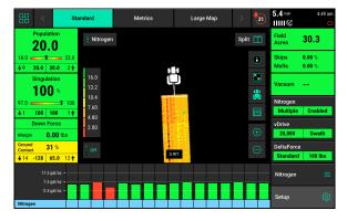
The control button (indicated by the product nickname that was selected during the setup process) will display the rate being commanded as well as the average rate being applied per acre. Pressing on this button will access the vApplyHD or FlowSense control page.
