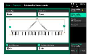
Measurement A - Wheel Distance: With the Sidedress bar lowered, measure the distance from the center of the drive wheels to the Pivot point. Enter this measurement in box A. Press the check mark button after entering the measurement.
