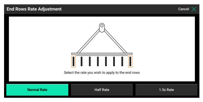
Effective Row Spacing and Effective Sidedress Bar Width are both automatically calculated from the number of Rows, Spacing, and Active Rows. If these are incorrect, they can be selected and a new value manually entered.
