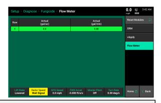
Flow (gal/min): Displays the flow measured in gallons/minute. Sensor Value (counts/sec): Displays the values that the flow meter is supplying to the 20|20.
