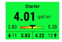
In the middle of the metric a rainbow chart that displays the planter average as a rectangle and each row as triangles. This chart is designed to give the operator a quick look at where all rows are at compared to the planter average. The low and high values on either end of the chart are determined by the Flow Alarm that is set in the Liquid Alerts.
