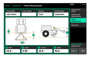
Measurements for implement mounted GPS systems are very similar to tractor mount GPS systems, except that measurements will be taken from the GPS output location on the implement instead of an output location on the tractor.
