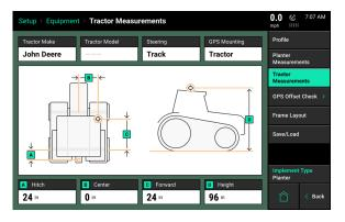
*C* - *Forward:* Measure from the track pivot to the GPS output location. Indicate if the GPS output location is in Front or Back of the pivot location.
