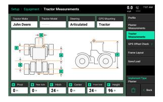
*D* - *Center:* Measure the distance from the center line of the tractor to the center of the GPS antenna. Then select if the GPS receiver is to the left or right side of the tractor's center line.
