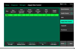
Flow (Gal/min): Displays the current status of the total flow of the system
