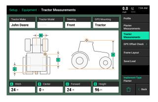
*C* - *Forward*: Measure the distance from the center of the rear axle to the center of the GPS antenna.
