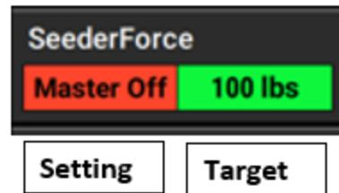
When the SeederForce system is enabled, the control button will display the Down Force Setting (Manual or Auto) and the SeederForce target value.
