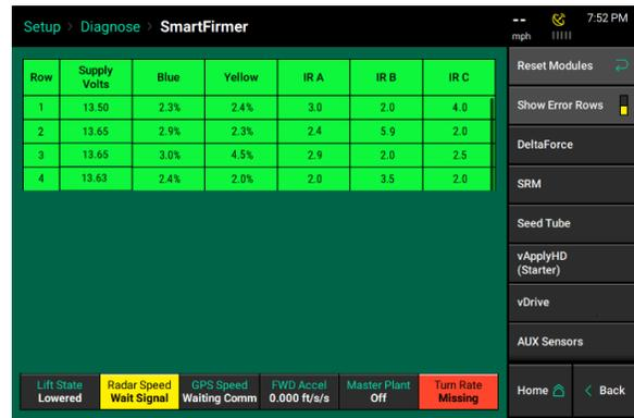
The screenshot shows the 'SmartFirmr' interface with a table of reflectance percentages. The table has 7 columns: Row, Supply Volts, Blue, Yellow, IR A, IR B, and IR C. The data is as follows:
