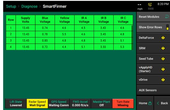
The screenshot shows the 'SmartFirmr' interface with a table of sensor voltages. The table has 7 columns: Row, Supply Volts, Blue Voltage, Yellow Voltage, IR A Voltage, IR B Voltage, and IR C Voltage. The data is as follows:
