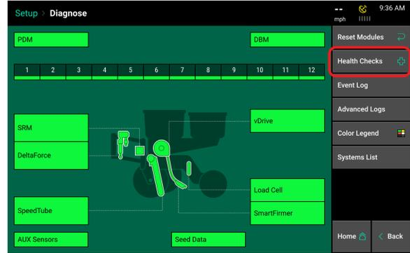
Select “Voltage/Current No Load” and follow the onscreen prompts for test requirements and to begin the test.
