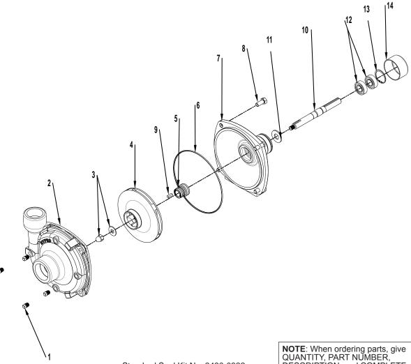
Silicon Carbide Seal Kit No. 3430-0589 consists of:
